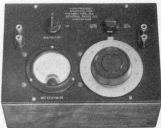
When supplied from a low-power oscillator, the audio-frequency microvolter enables known voltages between 1 volt and less than a microvolt to be obtained
